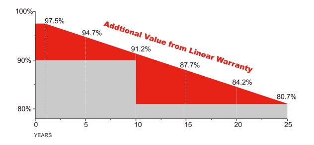
For Monocrystalline Products: less than 2.5% in the first year, thereafter less than 0.60% per year, ending with no less than 83.1% in the 25<sup>th</sup> year after the Warranty Start Date.
