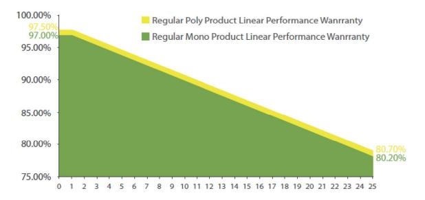
3). Double glass Poly product exhibits a power output no less than 97.5% of the nominal peak power specified on the respective datasheet or module label at STC within the first year from the "warranty start date", and power output declining by no more than 0.5% per year of the nominal peak power as specified on the respective datasheet at STC from the
