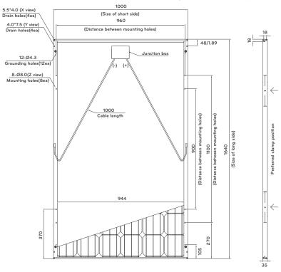
$<sup>\</sup>mbox{\ensuremath{^{\star}}}$  The distance between the center of the mounting/grounding holes
